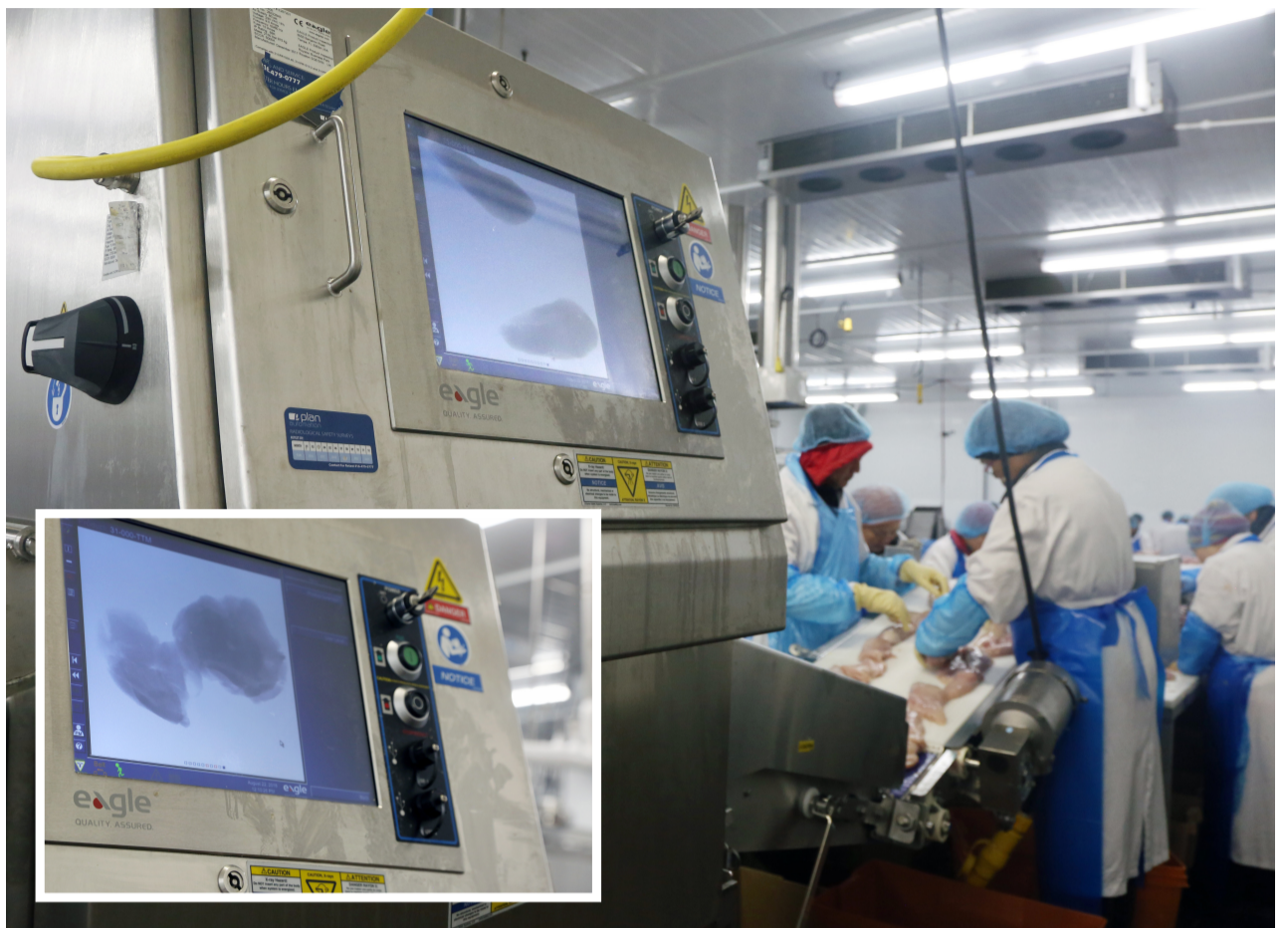
Designed to NAMI (North American Meat Institute) standards with hygienic construction and an IP69K rating for optimal protection against high-pressure and high-temperature washdowns, the Eagle RMI 400 system combines proprietary SimulTask PRO imaging software with a user-friendly touchscreen to enable highly accurate and reliable bone detection.
